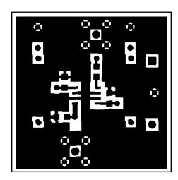
Figure 6: 730045 Component Side (top) Showing Ground Plane
